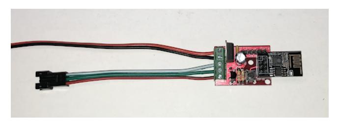
Step #9 - Insulate the extra power wires on the Pixel strip.
