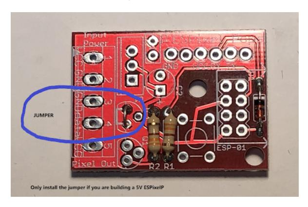
**Step #4** - Following the steps below, insert each part, solder it in place and snip off the extra leads. Below each set of steps is a picture showing the parts location:
