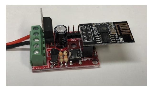
**Step #8** - Connect power and pixel connectors
