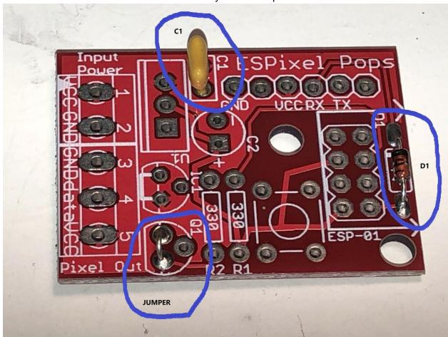
**Step #5** - Following the steps below, insert each part, solder it in place and snip off the extra leads. Below each set of steps is a picture showing the parts location:
