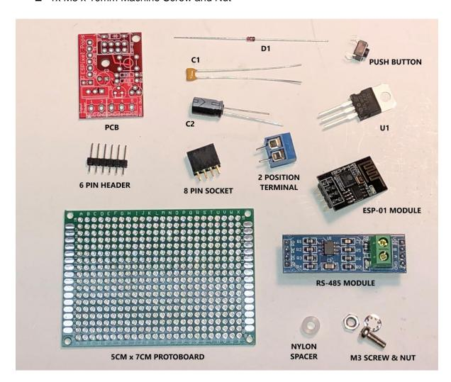
**Step #2** - Layout the PCB and RS-485 module on the protoboard to determine a location for the mounting screw. If you place the ESP-01 modules pins through the PCB socket holes you can align the board. You also want the PCB terminal strips to roughly line up with holes in the protoboard. Make a note of where these holes line up (here they are in the H row). Mark the ESPixelPOPs center mounting hole (just left of C2 below) on the protoboard (it will be a bit off center).
