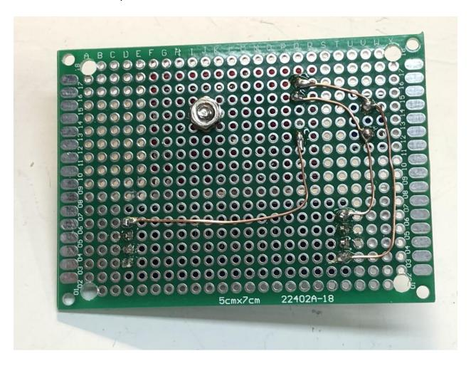
**Step #11** - Connect to power and a smoke test
