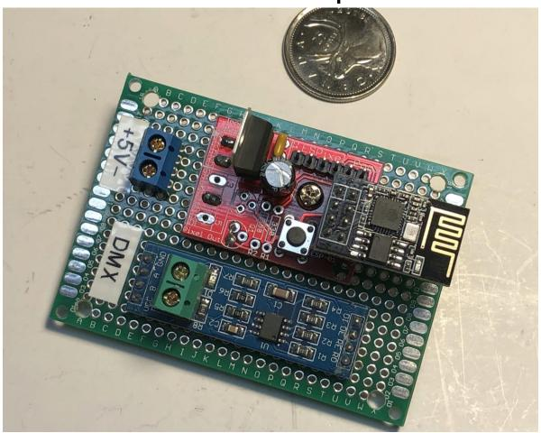
In this guide we will put together a DMX version of the ESPixelPOPs. This isn't for controlling Pixels but instead will output a DMX signal for use as an E1.31 to DMX bridge, capable of streaming one Universe of DMX data.
