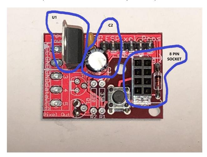
**Step #7** - This part is a bit tricky but you need to solder a short length of cut off lead into the terminal strip VCC, GND and DATA holes.
