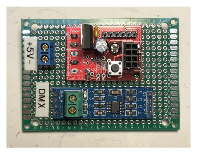
**Step #10** - Next we just need to do a bit of wiring to connect it all together. I use 24 gauge solid copper wire from Cat5 cabling that I have scrounged over the years.
