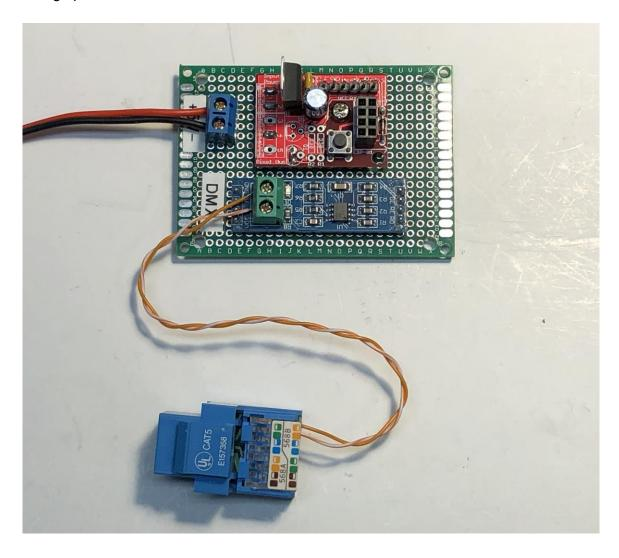
In the RJ-45 example above I have not connected the ground. If this is desired you can connect pin 7 (White/Brown) to the 5V power GND connection.
