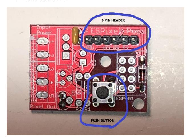
**Step #6** - Following the steps below, insert each part, solder it in place and snip off the extra leads. Below each set of steps is a picture showing the parts location:
