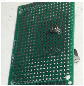
**Step #9** - Now install the remaining components on the protoboard. I find it best to just tack these in place with a bit of solder to ensure they don't move while we finish the wiring.
