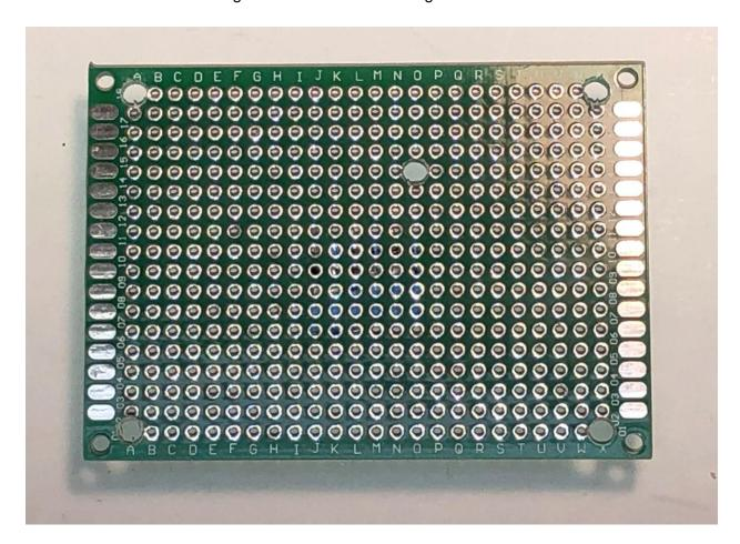
**Step #4** - Now start working on the PCB. Following the steps below, insert each part, solder it in place and snip off the extra leads. Below each set of steps is a picture showing the parts location:
