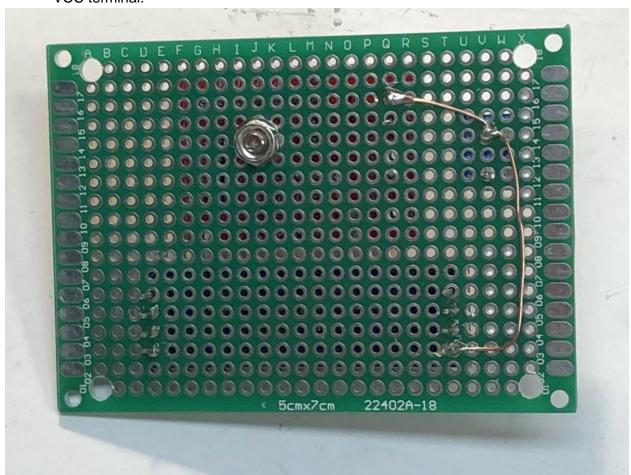
□ Connect GND from the power input terminal, to ESPixelPOP GND terminal & to RS-485 GND terminal.
