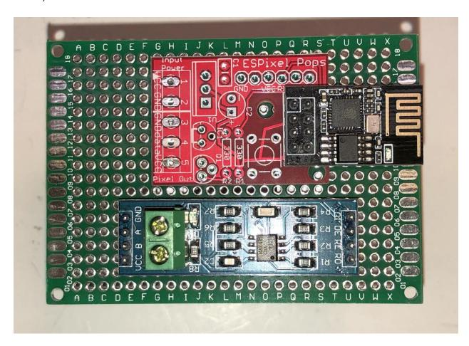
**Step #3** - Using a 1/8" bit drill out the mounting hole on the protoboard. I also drill a new mounting hole in each corner of the board as I find the existing ones in the protoboard are too small and too close to the edge to be able to drill out larger.
