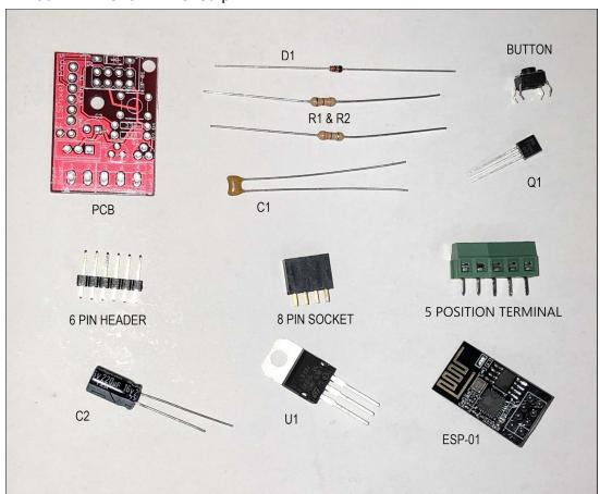
**Step #2** - Following the steps below insert each part, solder it in place and snip off the extra leads. Below each set of steps is a picture showing the parts location:
