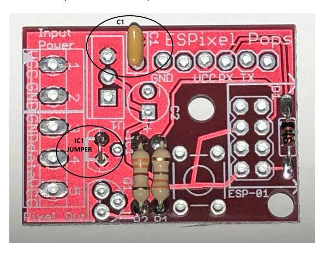
**Step #4** - Following the steps below insert each part, solder it in place and snip off the extra leads. Below each set of steps is a picture showing the parts location:
