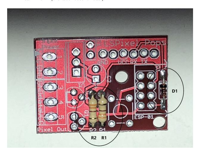
**Step #3** - Following the steps below insert each part, solder it in place and snip off the extra leads. Below each set of steps is a picture showing the parts location:
