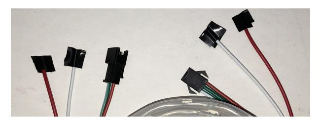
☐ Connect the input connector on the Pixel Strip (it will be on the end with the arrow facing into the strip) to the matching connector on the Pixel Strip Connector. It will only connect one way
