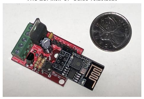
The ESPixelPOPs is a compact Wi-Fi based E1.31 (DMX over Ethernet) to Pixel (WS281x) controller that can handle up to 680 pixels (4 DMX Universes) of E1.31/sACN data. More information on ESPixel POPs can be found here:
